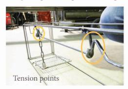
This is the proper trigger setting. With the trigger set there are no tension points to impede the trip pan.
