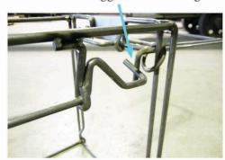
As you can see, when the trigger bar is set too high, it creates tension in the eye-loop and the plate won't trip.
