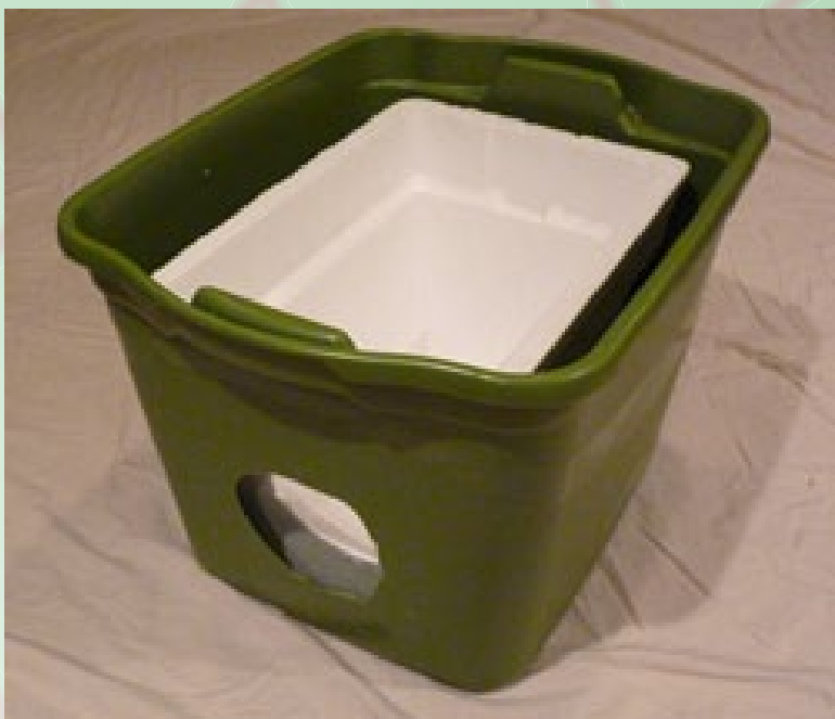
Step 2: Insert your Styrofoam cooler insulation and cut a matching 6" diameter hole to match the tote.
