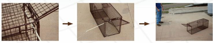
When the animal(s) enter the trap, pull the string to release the dowel and the trap door will close. You can then release the animal(s) by raising the rear sliding door, or by rolling the trap over to make the front door fall open.
